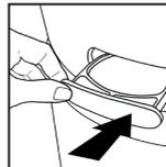
5. Place the oil tray back in its compartment and push to close. The scent will start automatically when the air purifier is turned on.
