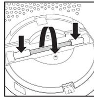
3. Gently push from the sides and rotate the UV-C bulb to remove.
