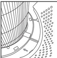
5. Place the tabs at the bottom of the grille cover into the base of the air purifier. Gently push the grille cover until it snaps into place.
