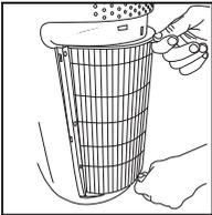
3. Pull the tabs to remove the old filter.
