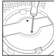
1. Unplug the air purifier and remove the HEPA-type filter. Using a Phillips-head screwdriver (not included), unscrew the 2 screws located on the UV-C bulb cover.
