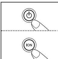
6. Plug the power cord into a standard AC outlet and press the power button. Press and hold the ioniser **ION** button for 3 seconds to reset the indicator.
