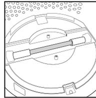
2. Remove the cover to expose the UV-C bulb.
